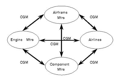
The ATA interchange profile for CGM has been very successful in providing the industry with a common method of delivering and interchanging technical illustrations. Several other industry groups have adopted this profile, and it was used as the baseline in the development of the WebCGM profile.
