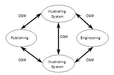
All interfaces beyond the illustrating system are controlled by CGM interchange. A single interpreter and a single generator filter is maintained, resulting in a more robust architecture. Changes to the illustrating system result in less development effort to support interchange.
